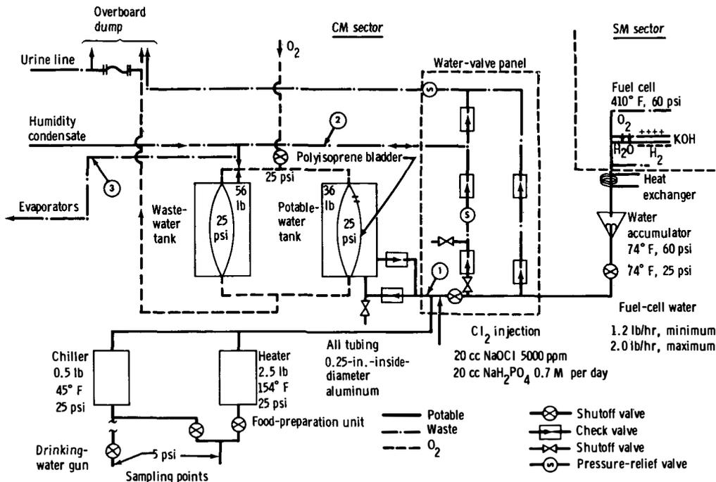
Figure 1. - Schematic of the CSM water management system.
