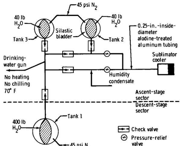
Figure 2. - Schematic of the LM water management system.
