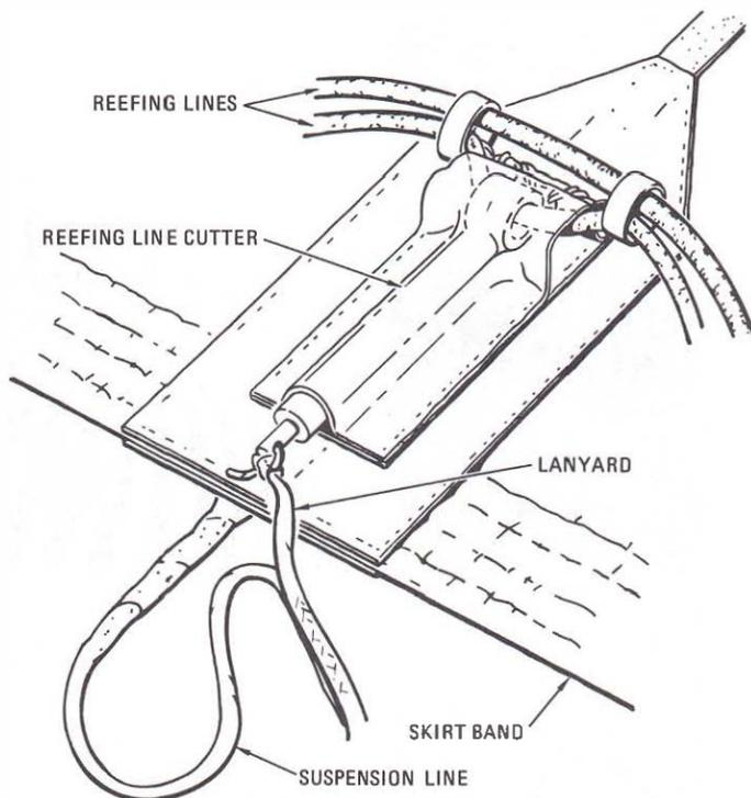
P-138 Reefing line cutter installation
