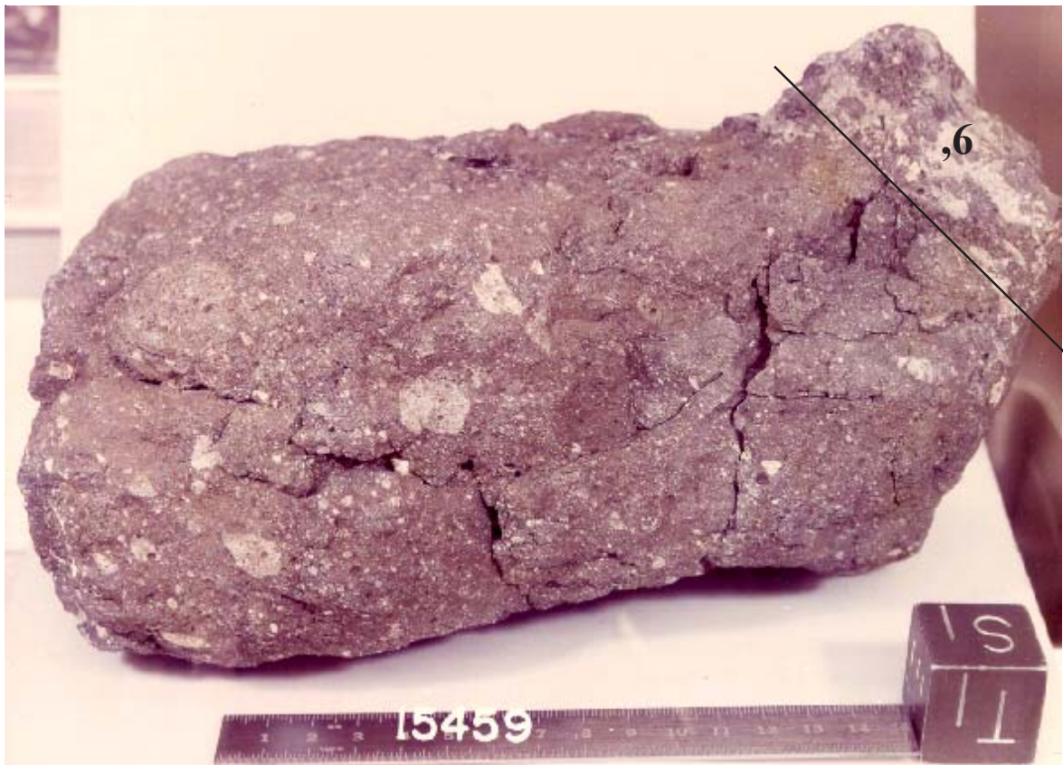
Figure 19: Photo of top side of 15459 showing zap pits, prominent clasts and marbled region on west end. NASA S75-32546. Cube is 1 inch. Location of ,6 used for public display is estimated.
