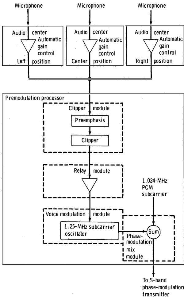
Figure 3. - Command module normal-voice signal flow.
