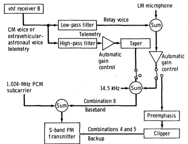
Figure 7. - Lunar module baseband- and backup-voice signal flow.
