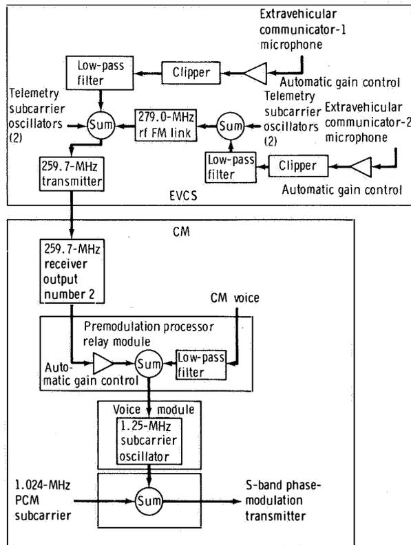
Figure 5. - Command module relay of EVCS signal flow.
