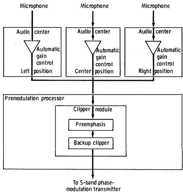
Figure 4. - Command module backup-voice signal flow.
