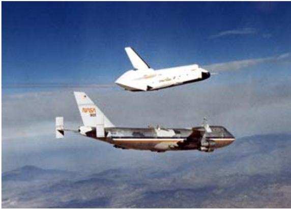
**The Space Shuttle prototype *Enterprise* flies free of NASA's 747 Shuttle Carrier Aircraft during an early Approach and Landing Test**
