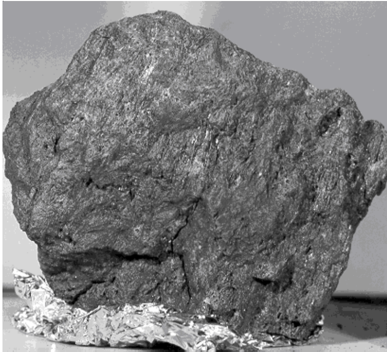
Figure 1: Photo of 15476 showing micrometeorite craters and underlying foliation caused by long pyroxene phenocrysts. Sample is about 8 cm across. NASA S71-46905.
